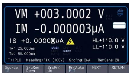
Source voltage (VS), source current (IS), limit values (HL/LL), measured voltage (VM) and measurement current (IM) are displayed. Voltage and current can be measured simultaneously.
