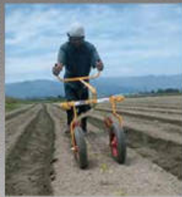
Onion transplanter Model number P047-B Overall height 800 mm Inside Diameter Φ25 mm
