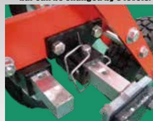
The width of the GL horizontal bar can be changed by 6 levels.
