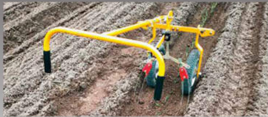
Sugar beet transplanter Model number P047-A Overall height 870 mm Inside Diameter Φ38 mm
