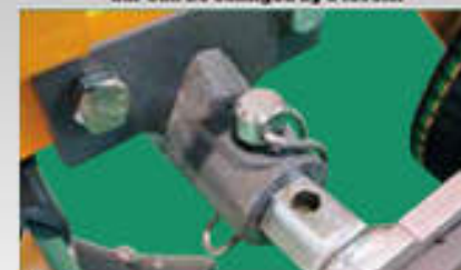
The width of the S3 horizontal bar can be changed by 6 levels.
