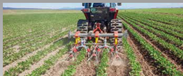
The width of the GL horizontal bar can be changed by 6 levels.
